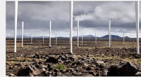
A Spanish startup designed a new wind turbine using a vibrating upright cylinder to catch the wind, a.k.a. "the Skybrator." No blades, gears, or oil needed; only vortex shedding as the swaying is converted by an alternator into electricity: smaller, queter, and less invaries.
