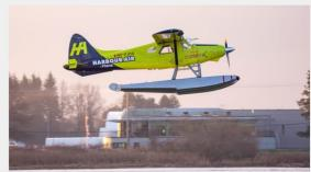
An historic first short-haul all-electric test airplane stayed aloft for 3 minutes above the Fraser River east of Vancouver. The joint Harbour Air and MagniX 11 e-plane was powered by NASA-approved lithium-ion batteries and a standard-design though lightweight electric motor. As batteries improve, the sky is literally the limit.
