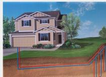
A neighbourhood Montreal co-op began heating 7 homes retrofitted with geothermal heat pumps (aka ground source heat pumps or geoexchange systems). To reduce costs and comply with laws, 8 150-m-deep geothermal wells were dug in a private backyard rather than a public alleways, and are shared. The goal is to connect 50 homes. AC is also svalable.
