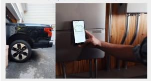
Vehicle-to-grid technology (YZG) or directional charging counters intermittency of wind and solar, requiring one-third of drivers to opt in. Baltimore Gas and Electric Company, Sunrun, and Ford are part of the first US residential V2G project using home solar and Ford's F150 Lightning EV, whose batteries are 10 x a typical home pack and 90% dormant.
